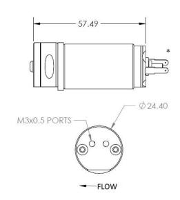
\*Positive and negative solder tabs on motor (for 20 AWG wires)
